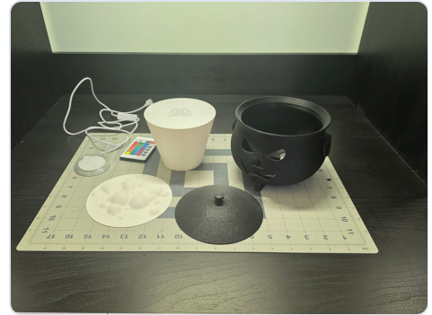
Four printed parts and one puck light. The white cone is the diffuser; the disc of domes is the brew. The light, the remote and the lead are the parts you buy.
