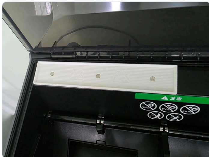
One rail down, aligned to the front edge of the lip.
