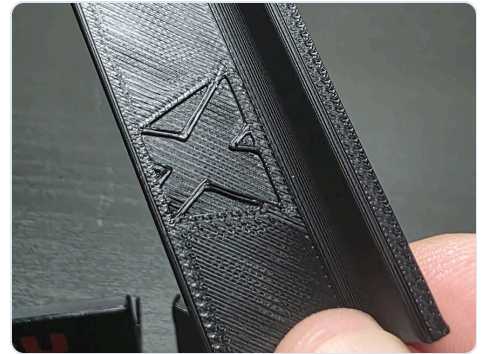
The back. That L-shaped channel is the whole mounting system — it hooks the front edge and gravity does the rest.
