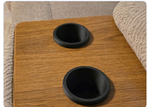
Seated in the arm caddy. The textured lip covers the cut edge of the opening.
