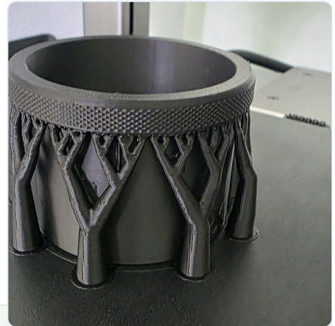
Straight off the plate. The tree supports fan out under the lip — that is the 9.26 g the slicer quoted.
