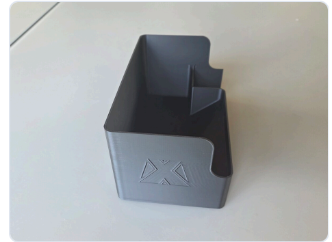
Looking in: the internal wall and the stepped rear cutout are part of the same shell.
