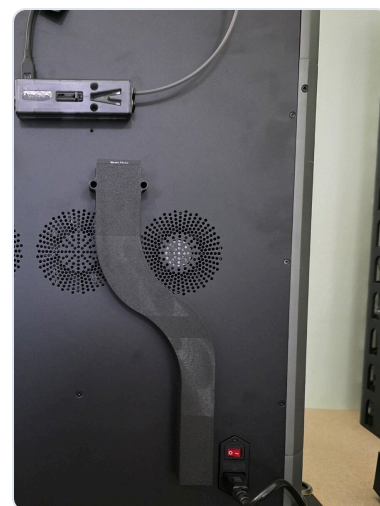
Installed: from the waste port down past the fans.
