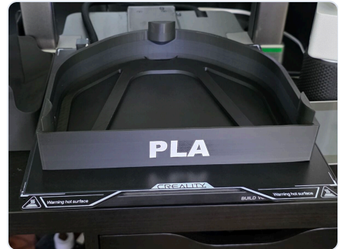
Off the plate in one piece. The auto brim is the only thing to remove.
