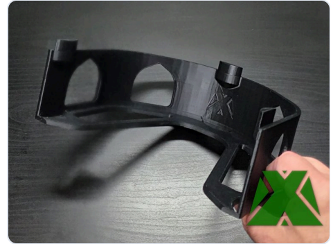
One unit. The pegs on the top edge are what the next shelf sits on.
