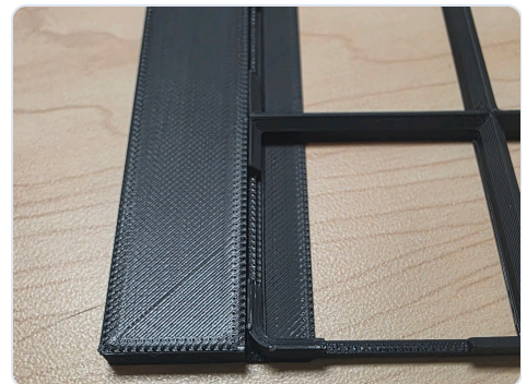
Lip under the plate, top level with the grid.
