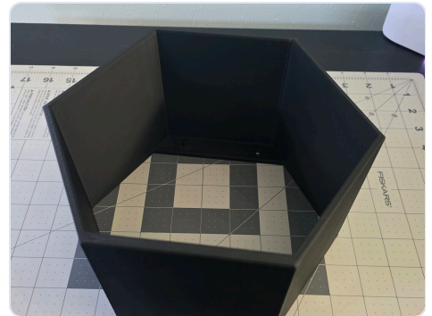
219 mm across the points, 120 mm deep. The mounting plate is the band across the far top facet.
