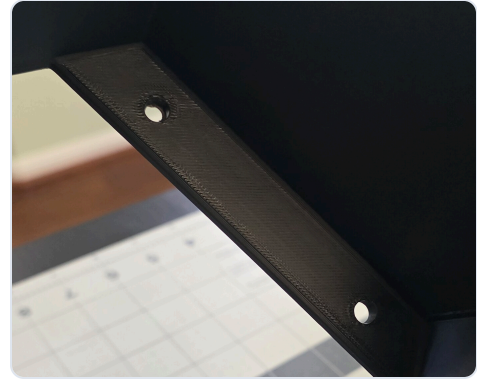
The mounting plate, printed flat on the bed. Those diagonal lines are its solid top surface — no supports touch it.
