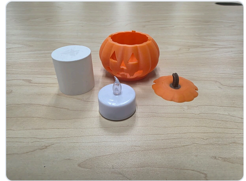
Three printed parts and one battery tea light. The white cylinder is the diffuser.
