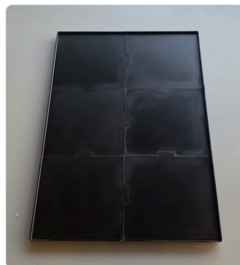
Six panels, glued into one tray. The seams are the thin lines with the dovetail steps.
